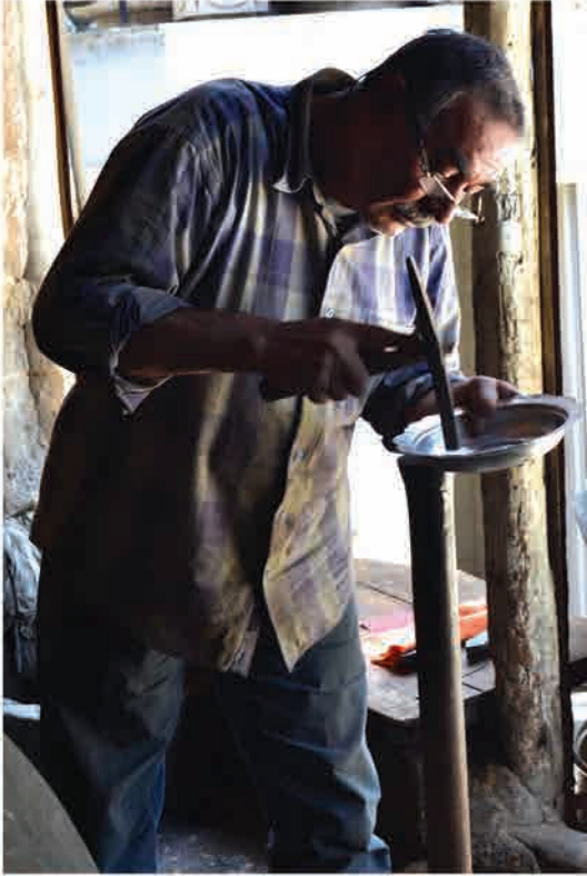
Master Mehmet Elmas while Straightening Copper / Southern Aegean Development Agency Archive
