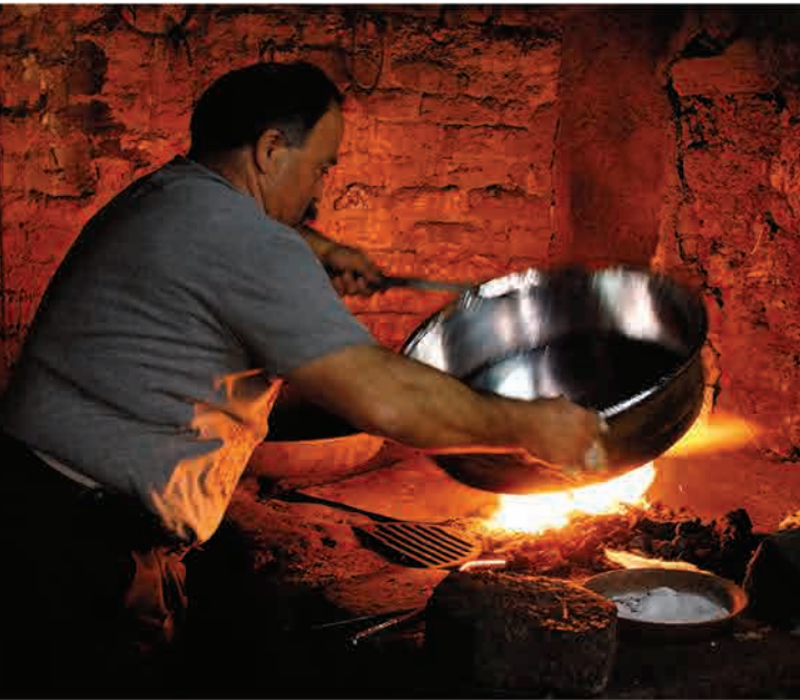
Copper while Tin Plating / Ümit Özgür
