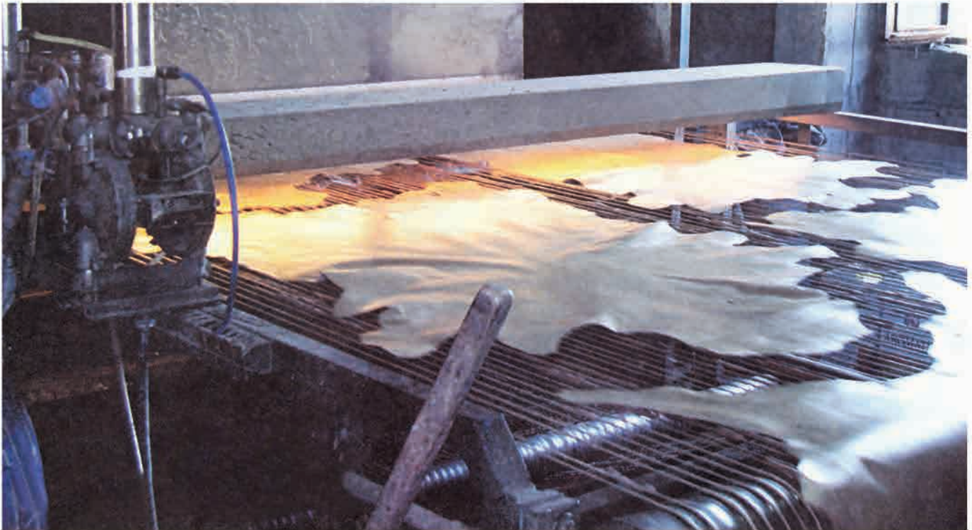
Leathers Dyed at Tunnel Exit / Archive of Denizli Leather Specialization Organized Industrial Zone Directorate
