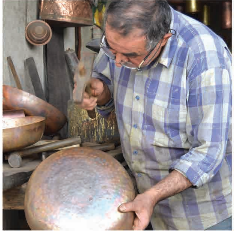
Master Mehmet Elmas while Straightening Copper / Southern Aegean Development Agency Archive
